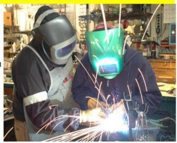
If you can design a sheet metal component which can be manufactured in one piece this is nearly always the best approach. However, you may have to design a component that has two or more gauges of sheet metal, shapes that would be materially inefficient to be CNC punched from one part, impossible to be manufactured as one or needing water tight joints. Welding enables you to bring these parts cut from sheet metal together into one fabrication.
