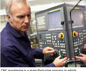
CNC machining is a manufacturing process in which pre-programmed computer software dictates the movement of factory tools and machinery. The process can be used to control a range of complex machinery, from grinders and lathes to mills and routers. With CNC machining, three-dimensional cutting tasks can be accomplished in a single set of prompts.
