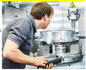
Machining techniques are often divided into four categories, and may be used together to produce a single product. Drilling is one of the most basic types of machining. Turning is another form of machining used to shape metal. Milling uses metal bits to cut material out of the surface or face of an object. Grinding is a simple process which involves using a stone-grinding wheel to shape or polish metal.
